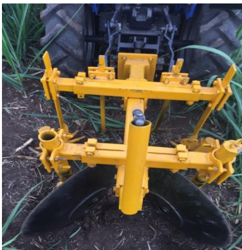
Fig. 8 Weed extractor on the field
