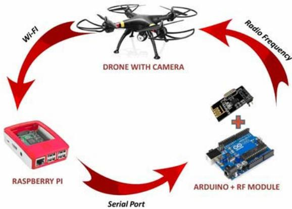
Figure 5: Communication scheme for the flight control of the drone.
