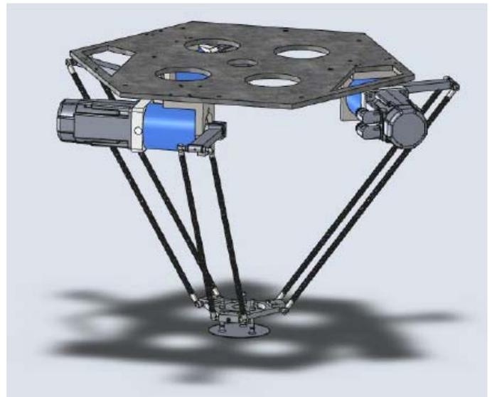
Figure 6: A 3D rendering of the Delta Robot.
