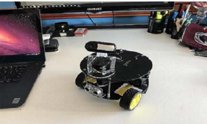
Figure 4: Three wheel robot with camera and proximity sensor.
