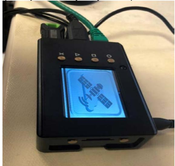
Figure 7: SatCOMM Relay Controller (SCR) Version 1
